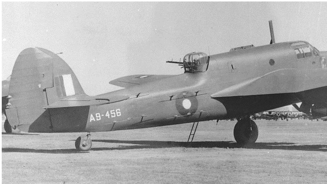
The starboard-side Search Array on a Beaufort VIII with seven of the eight directional antennas visible. This aircraft is in overall Foliage Green. [Peter Jackson Collection, State Library of SA image PRG 1614/2/49].
