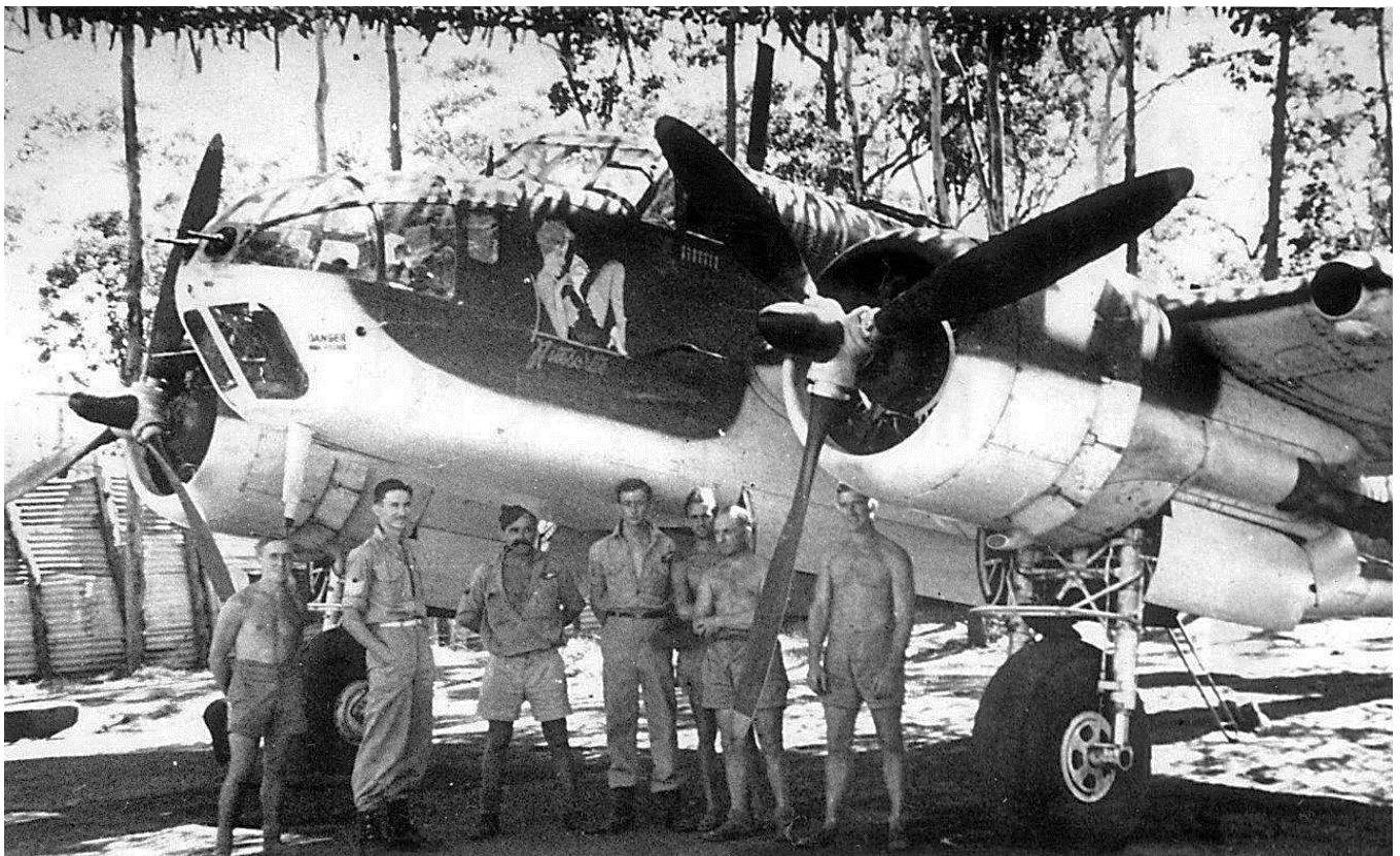
Forward quarter view of 2SQN's A9-576/KO-Z. The name, nose art and bomb log are visible from this aspect; also the typical style ASV Homing array – no Yagi aerials under the wings. [Image via Kas Grigonis, ADF-Serials facebook page].
